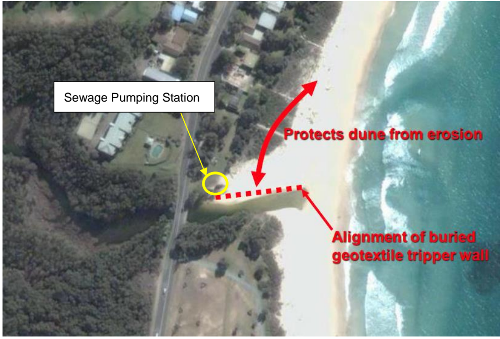
Figure 3 – Suggested alignment for buried tripper wall north of Blackwater Creek showing location of Sewage Pumping Station (SMEC 2011)
