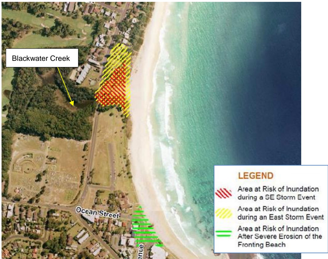
Figure 2 – Area subject to coastal inundation north of Blackwater Creek prior to construction of tripper wall (SMEC 2011)
